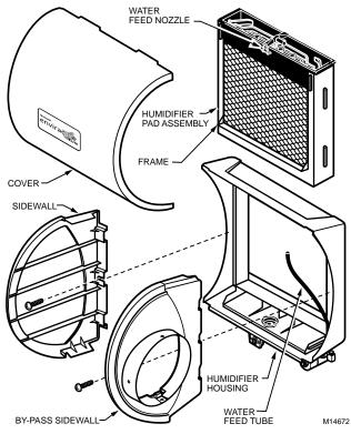
Fig. 4. Humidifier components.
